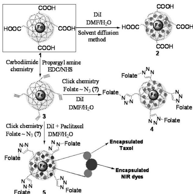
**Scheme 1.** Schematic representation of the synthesis of theranostics and multimodal IONPs. Click chemistry and carbodiimide chemistry have been used for the synthesis of a library of functional IONPs. NIR dyes and paclitaxel co-encapsulated IONPs were prepared in water using the modified solvent diffusion method (see Supporting Information 1 and 2 for detailed synthetic procedures).
